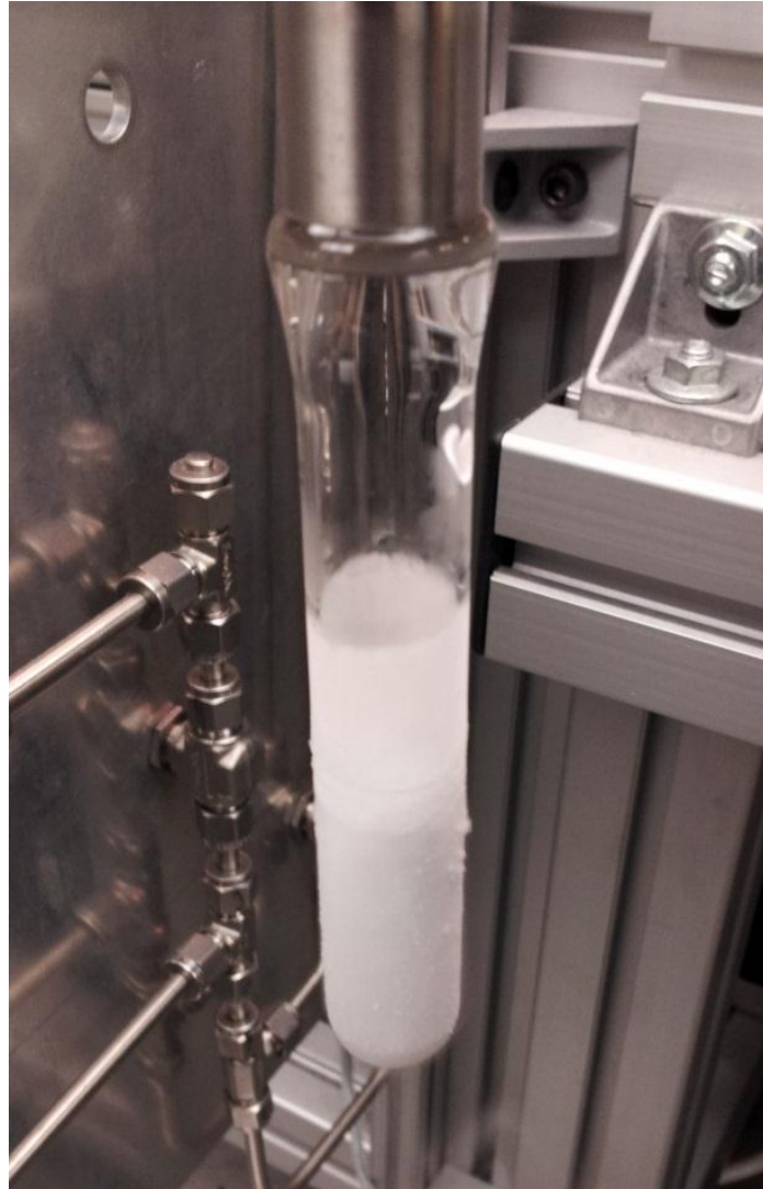
Figure 20: Frozen acetone while evacuating the vial.
